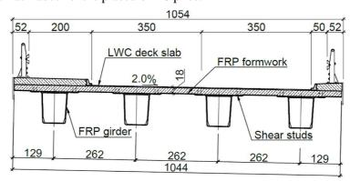
Fig. 7. Cross section of the hybrid bridge in Błażowa, Poland [cm]
