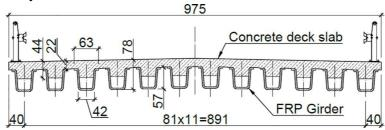
Fig. 3. Cross section of the bridge span in San Patricio Country, USA [cm]
